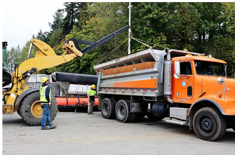
Street Maintenance crews place a sanding unit into the bed of a plow truck during their winter preparations in October.
